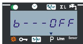
It is VERY important that this is set to OFF. If the display indicates anything else then use the **Set** arrow buttons to ensure that it is set to OFF. *Explanation: This facility can force a regeneration, regardless of reserve volume allowances used in delayed meter initiation applications. It is not normally relevant to simple installations.*
