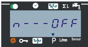
It is VERY important that this is set to OFF. If the display indicates anything else then use the **Set** arrow buttons to ensure that it is set to OFF. *Explanation: This provides for the operation of an auxiliary output relay which is not normally relevant to simple installations.*
