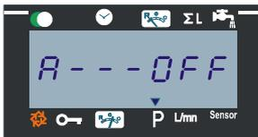
It is VERY important that this is set to OFF. If the display indicates anything else then use the **Set** arrow buttons to ensure that it is set to OFF. *Explanation: This facility can force a regeneration, regardless of volume throughput or programmed time frequency. It is not normally relevant to simple installations.*
