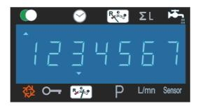
Water flow throught the system is indicated by the meter arrow flashing in a direct relationship to the flow rate. As treated water is produced, the volume remaining display will count down towards zero. On reaching that point, the recovery process will commence. The volume unit of measurement is m<sup>3</sup>.
