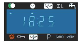
In normal operation the time of day (24 hour format) will be displayed at all times. The control will operate normally until the point when the recovery initiation parameters have been met. The recovery process will then commence.
