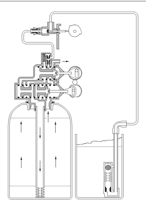
Softened water from the second pressure vessel flows around the lower piston, around the upper piston and exits into the bottom of the first vessel via the bottom screen. The resin bed is expanded by the upflow of water, which then exits the valve via the upper piston and flows to drain.
