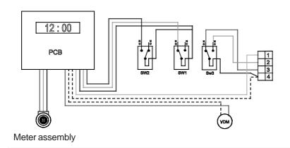
Electrical supply connections: 24vac 50 Hz. 10 Va Negative to TERMINAL 1 Positive to TERMINAL 4
