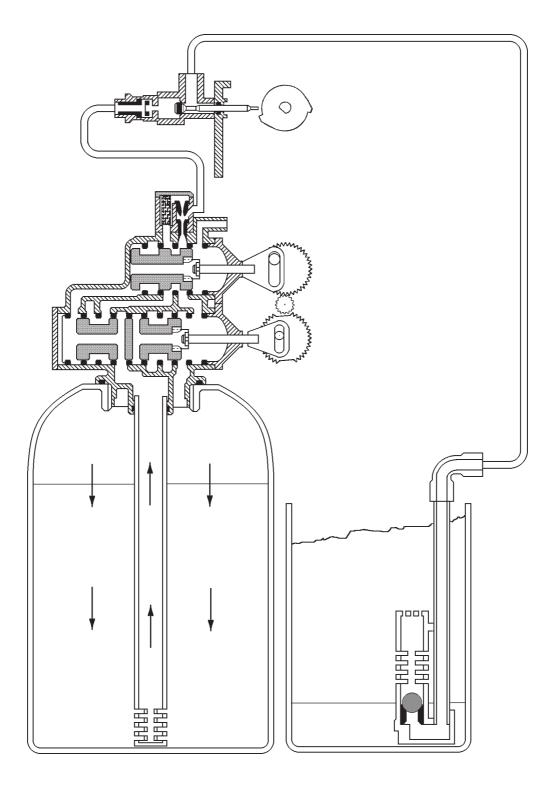
Softened water from the second pressure vessel flows around the lower piston, around the upper piston & down through the resin in the first vessel. The rinse water exits the first vessel via the bottom screen. It flows up the centre tube, through the bore of the lower piston and up into the upper valve section where it exits via the bore of the upper piston to drain.
