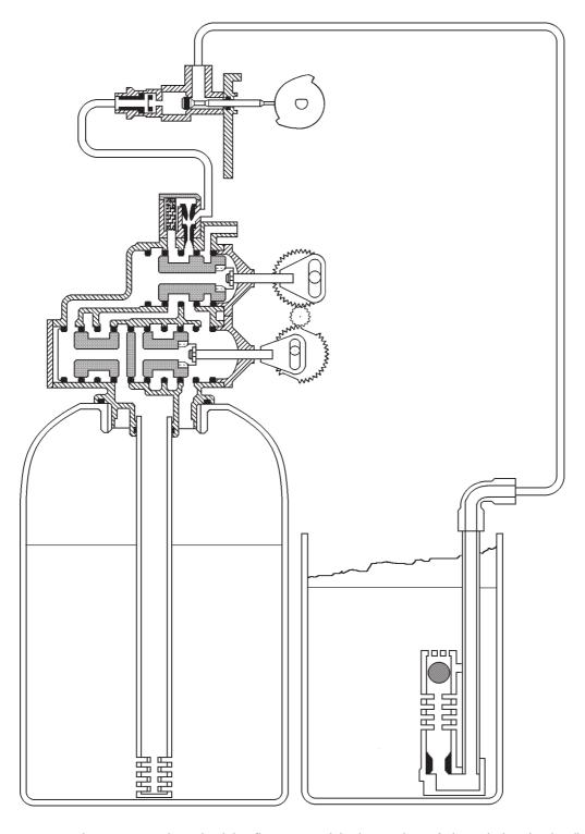
Hard water enters the system at the valve inlet, flows around the lower piston & through the pipe leading to the second vessel, passing through the resin in the second vessel. Softened water exits via the bottom collector system in the second vessel. It transfers via the connecting pipe to the valve, flows around the lower piston and flows to service via the water meter. The first resin vessel is out of the service flow path & is ready for regeneration.
