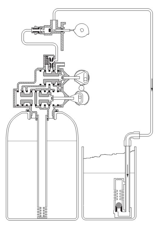
Softened water from the second pressure vessel flows around the lower piston, around the upper piston & into the ejector housing. The flow rate is regulated by a flow orifice as the softened water exits via the brine valve and into the brine tank. In addition to refilling the brine tank, the softened water also flushes the brine system and resets the air check ball. No water flows through the first vessel at this stage.
