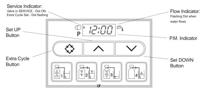
Push either the UP or DOWN set button once to adjust the Time of DAY display by one digit. Push and HOLD either the UP or DOWN set button to adjust the Time of Day display by multiple digits
