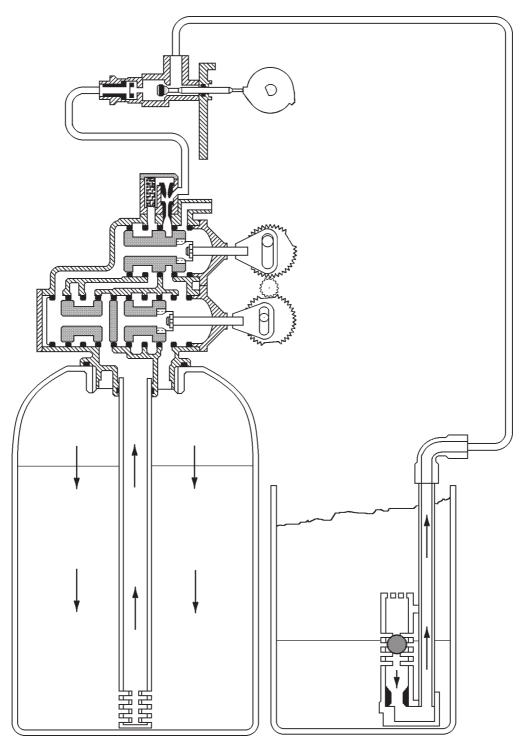
Softened water from the second pressure vessel flows around the lower piston, around the upper piston & into the ejector housing. As it passes through the ejector nozzle, a vacuum is generated which draws brine up from the brine tank. Brine flows around the upper piston, down through the resin bed and exits via the bottom screen. It flows up the centre tube, through the bore of the lower piston and up into the upper valve section where it exits via the bore of the upper piston to drain.
