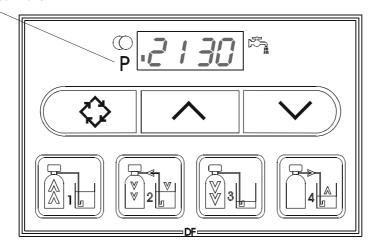
1. The first option setting display that appears in the Programme Mode is Treated Water Capacity. Using the Set UP or DOWN button, set the display to the capacity of the system in LITRES or CUBIC METRES. For example, in LITRES:
