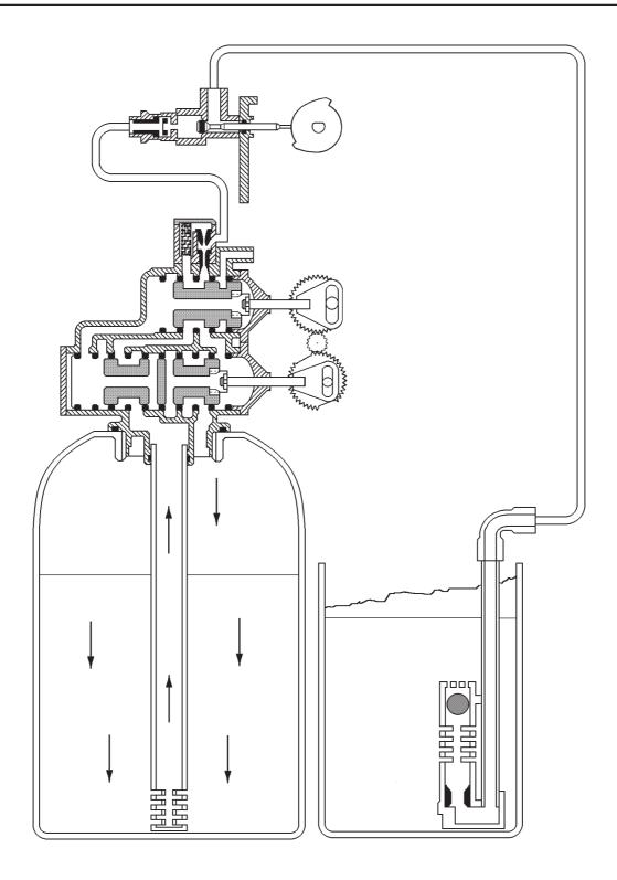
Hard water enters the system at the valve inlet, flows around the lower piston & down through the resin in the first pressure vessel. Softened water exits via the bottom collector system in the resin vessel, flows around the lower piston and flows to service via the system water meter. The second resin vessel is regenerated & on standby.
