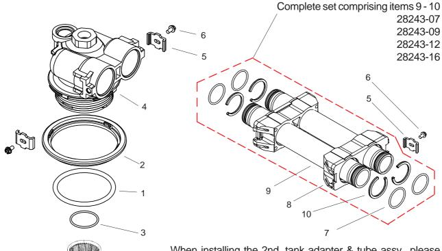
When installing the 2nd. tank adapter & tube assy., please remember that the mounting clip screws only need to be secured against the clip.
